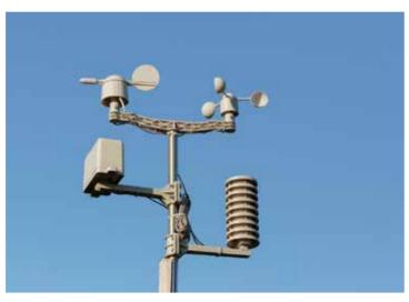
A weather station comprising of sensors for wind speed, wind direction, rain and temperature. In July 2017, the African Climate Policy Centre launched the second phase of the Weather and Climate Information Services for Africa (WISER), to be implemented within a span of three years. Photo Courtesy
